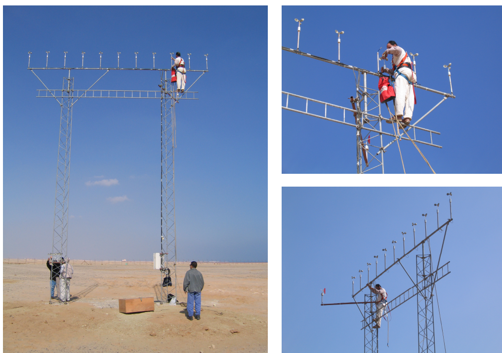
Figure C-1. Cup anemometer calibration facility at Hurghada WETC: upwind fetch to the NW (left) and details of the cup anemometer set-up (right).
